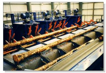
High capacity cross-cutting line for long poles
